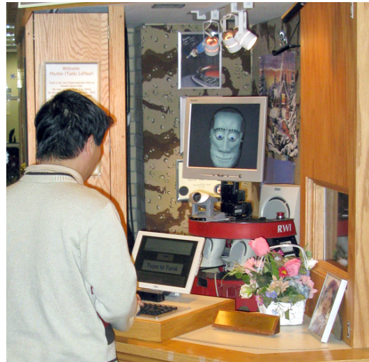
Figure 1. A photo of Roboceptionist, a receptionist robot located in a high-traffic entrance area in an academic building.
