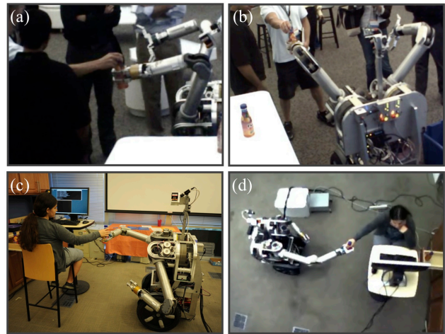
Figure 1: HERB (Home Exploring Robotic Butler) handing over a drink (a-b) during a public demonstration and (c-d) during our experiment for investigating effects of spatial and temporal contrast.
