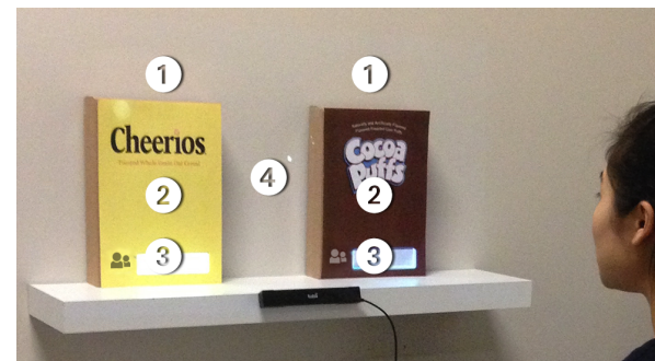
Figure 1. Interactive social shopping shelf: (1) the top: collective in-store gaze and purchase data, (2) the middle: an animation expressing ingredients, (3) the bottom: comments from a social network service and (4) information projection in the between the product: nutritional comparisons with adjacent products. Copyrights of the logos are held by General Mills.
